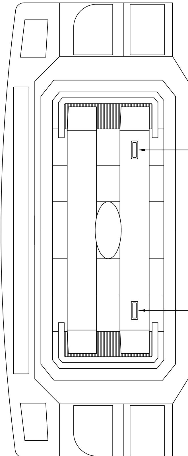
A. MODEL # LINZ6A. LIGHTS SHALL BE MOUNTED FLUSH OR PROTRUDING FROM GRILL. LIGHTS MOUNTED BEHIND GRILL ARE UNACCEPTABLE.
